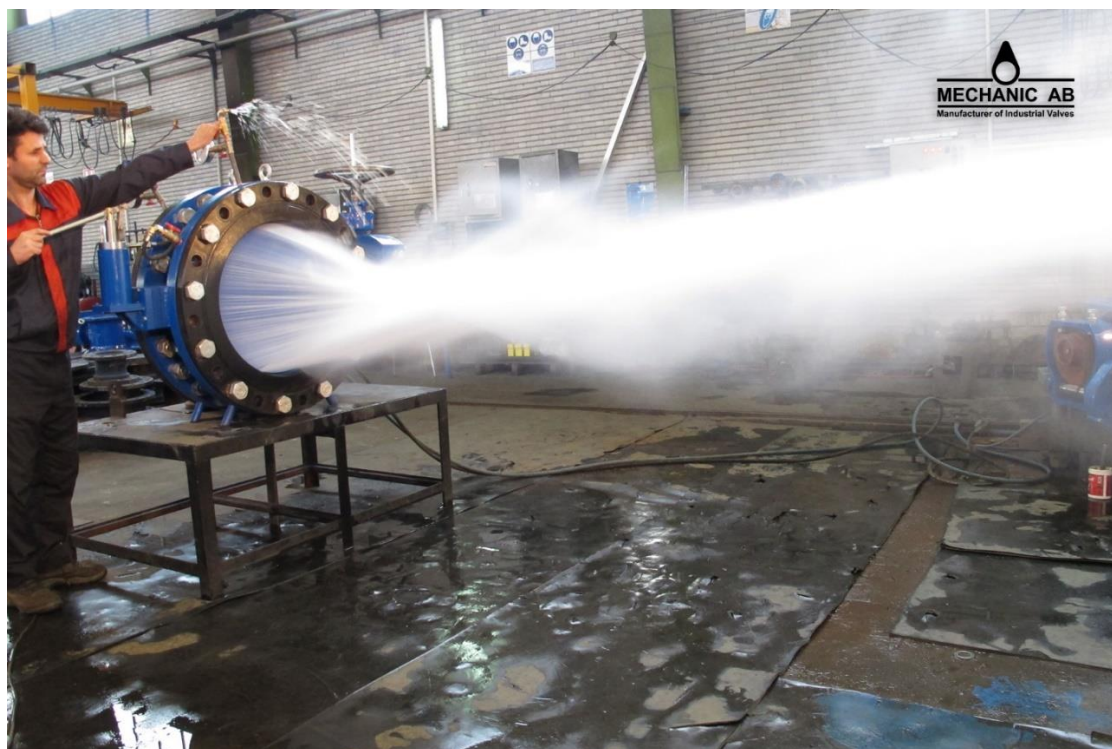
T-Butterfly Valve Hydro static test
